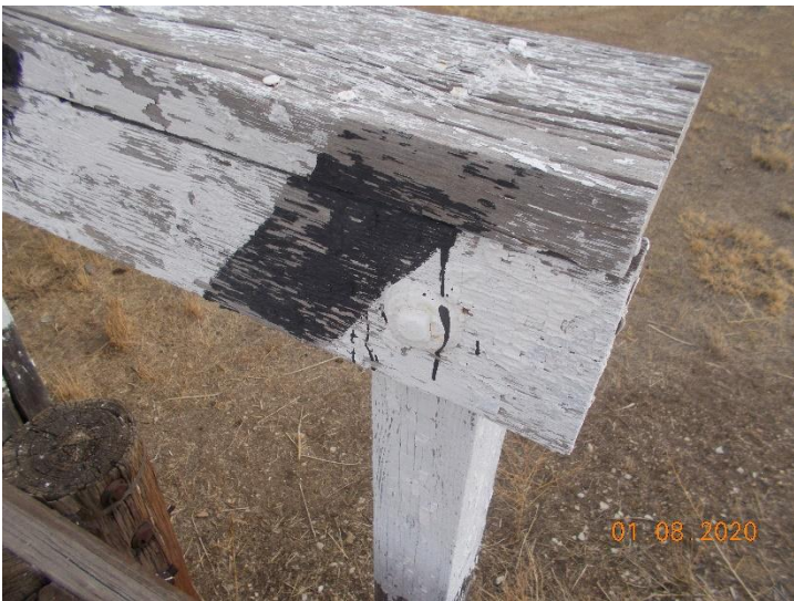
Paint sample M-21-J-LP01. The white paint is considered as lead containing paint.
